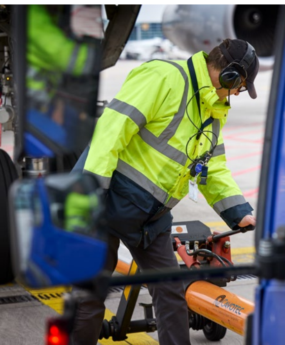
The ramp agent connects the aircraft to the pushback tug, also known as the "pusher", which then pushes the plane out to the taxiway. Afterwards, the ramp agent notifies the pilot and disconnects the cockpit from the DECT radio network - and from the pusher.
