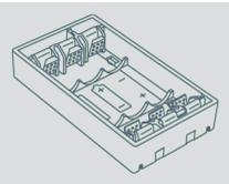
NiMH batteries or alkaline batteries can be used in the AAA adapters. The use of NiMH batteries is recommended.
