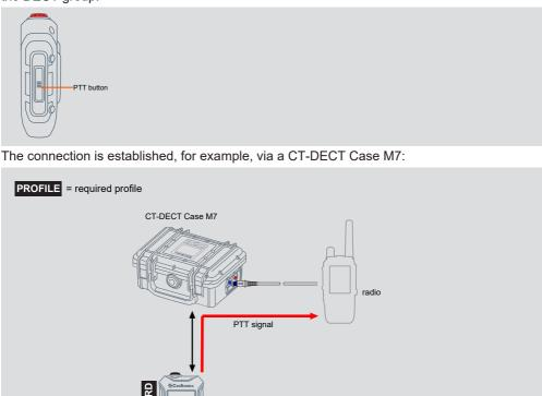
As long as the PTT button is pressed, the user can speak into the radio circuit. Meanwhile, the user continues to hear the DECT group.
