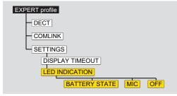
The default setting is BATTERY STATE. A change is retained even after restart.
