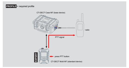
As long as the PTT button is pressed, the user can speak into the radio circuit. Meanwhile, the user continues to hear the DECT group.
