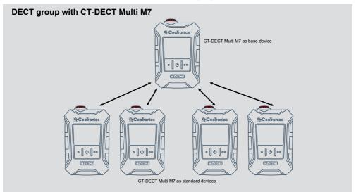
Depending on the software it is equipped with, the CT-DECT Multi M7 offers various profiles made for different use cases and roles.
