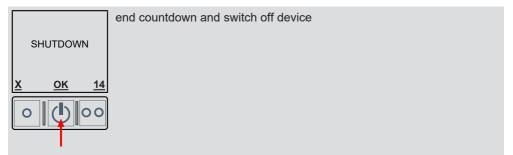
To cancel the countdown, either disconnect the adapter cable from the CT-DECT Multi M7 or press the left button. The device remains switched on and is powered by the internal battery.
