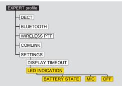
The default setting is BATTERY STATE. A change is retained even after restart.
