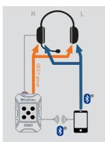
When set to ON, all sources (DECT group and Bluetooth® connection) are played back on both earpieces of the headset. It does not matter whether only one source or several sources are active.
