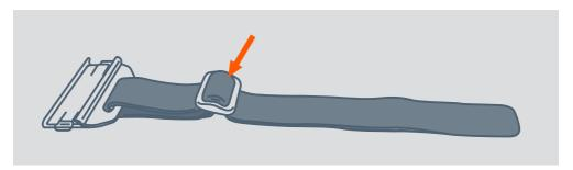
Guide the end of the Velcro strap through the holder and adjust to the correct size.
