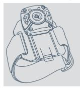
If using two CT-Wireless PTT MIL, also slide the second device into the holder. To remove, push the locking mechanism (arrow) downwards and slide the CT-Wireless PTT MIL out of the holder.
