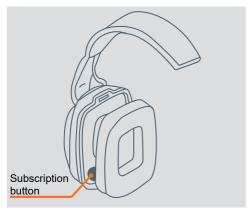
Press and hold the subscription button on the headset. While holding the subscription button pressed, switch on the headset with the On/Off button and volume control (rotary knob). After the headset switches on, keep the subscription button pressed for at least another 2 seconds until you hear a falling sequence of tones. Then release the subscription button.
