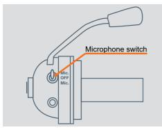
**Middle setting "OFF" (receive):** The headset microphone is switched off. You can only receive.
