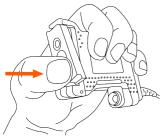
2. When opening the cover, make sure that the opening of the battery compartment is not facing downwards to prevent the battery pack / adapter from falling out.
